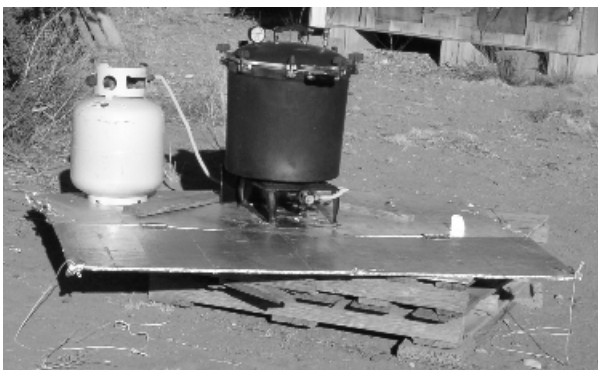
Fig. 2 Hood and Rear Reflector Removed. Base Reflector pivots on platform. Sterilizer at solar focus, over Pivot Pin
