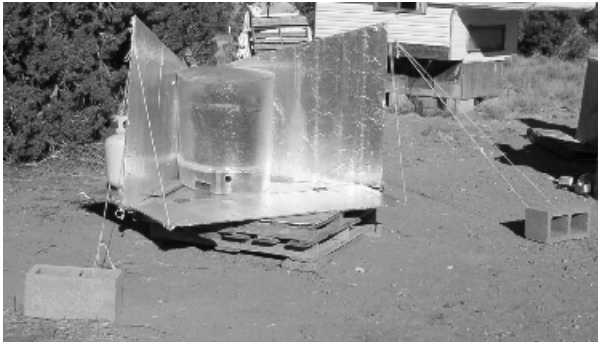
Fig.1 Hybrid Autoclave in Solar Operation. Low sun elevation configuration, Rear Reflectors vertical, Front Reflector horizontal. Unit pivoted toward sun.
