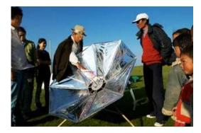
Portable parabolic solar cookers made of bamboo, yak wool, and Mylar are being developed by <u>One Earth</u> <u>Designs</u> for use by herding communities in the Himalayas.
