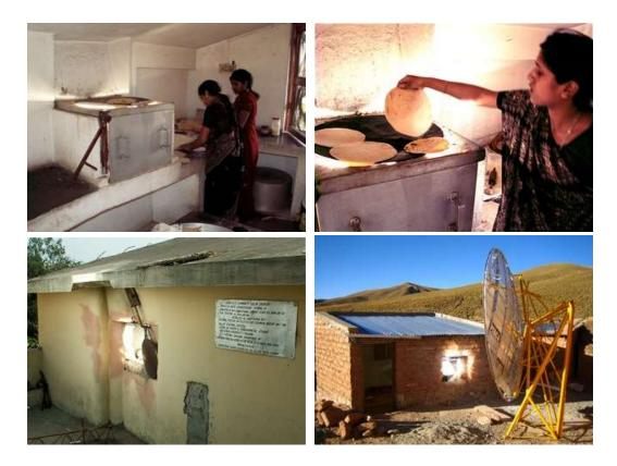
One of the Scheffler reflectors at Barli Institute <u>heats a storage unit</u>, which allows cooking at night.
